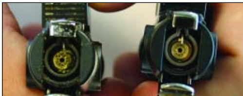
Clogged Flame Holes
