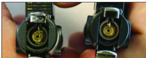
Clogged Flame Holes
