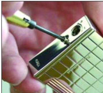
1. Unscrew the screw which holds the bottom cover to the gas tank.
