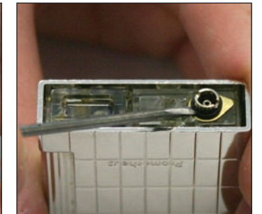
3. Remove the O-Ring from the Flame Height Adjuster.
