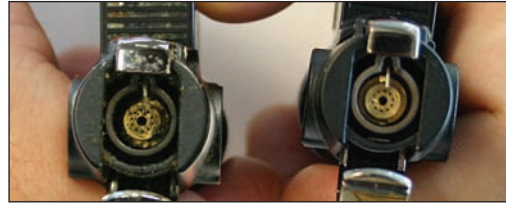
Clogged Flame Holes Properly Maintained
