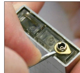
4. Remove the Stopper below the O-Ring.
