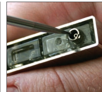
5. Turn the Flame Height Adjuster by a quarter turn at a time to the desired level.
